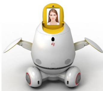
Slika 11. Engkey robot (Robotics Today, Engkey, 2018)
